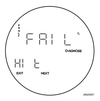
Figure 6-8. Fault 4, High Probe Temperature
